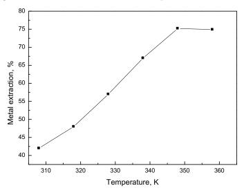
Fig. 2. Effect of temperature on the leaching efficiency of Al(III)
