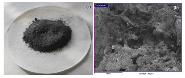
Fig. 1. Milled aluminum dross (a) SEM micrograph of the aluminum dross (b)
